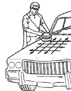
5. Work next on smaller surfaces (doors etc.) Always keep the mains lead over the shoulder or let it hang to the ground when working on a vertical surface making sure it is well clear of the moving polishing head. For less accessible surfaces (such as wing mirrors, door handles) remove the polishing bonnet and polish these areas by hand (see dia 5).
