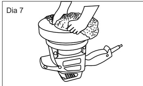
7. Use long, sweeping strokes in a criss-cross pattern to bring out the shine. Do not press hard. Let the polisher do the work (see dia 8).
