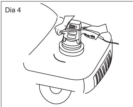
4. Hold extension lead over shoulder and do flat surfaces first ie: bonnet boot and roof. Cover areas quickly with broad sweeping strokes in a criss-cross pattern. Do not press down on polisher. The machine's action, not pressure, does the best job (see dia 5).
