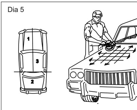
5. Work next on smaller surfaces (doors etc.) Always keep the mains lead over the shoulder or let it hang to the ground when working on a vertical surface making sure it is well clear of the moving polishing head. For less accessible surfaces (such as wing mirrors, door handles) remove the polishing bonnet and polish these areas by hand (see dia 6).
