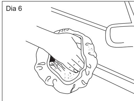
6. Finally remove the terry-cloth application bonnet and fit the synthetic wool polishing bonnet onto the polisher, (see dia 7).
