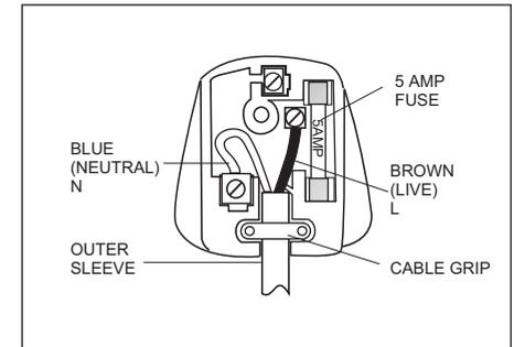
**Note** If a moulded plug is fitted and has to be removed take great care in disposing of the plug and severed cable, it must be destroyed to prevent engaging into a socket.
