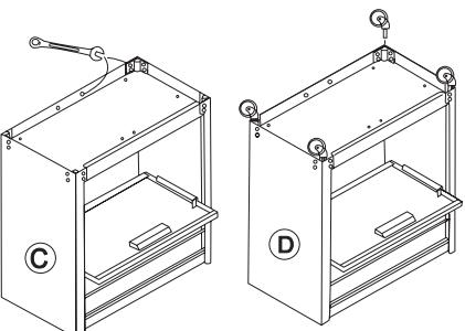
**Fit the caster brackets to the base of the cabinet with nuts & bolts supplied. Then insert castors (Tools not included for assembly).**
