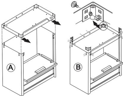
Carefully lay the cabinet on its top and refit base.
