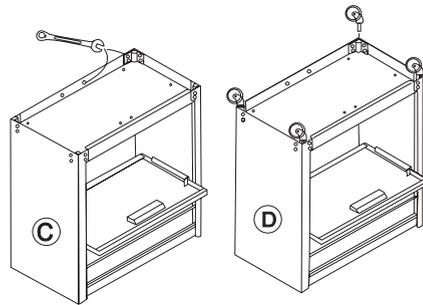
Fit the castor brackets to the base of the cabinet with nuts & bolts supplied. Then insert castors (Tools not included for assembly).
