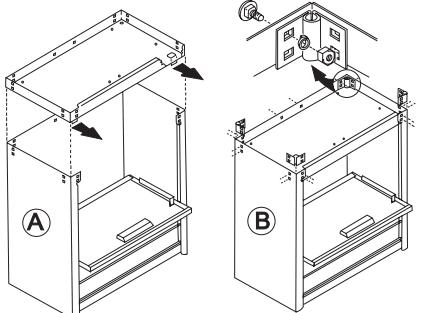
**Carefully lay the cabinet on its top and refit base.**
