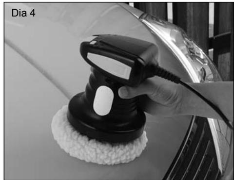
4. Hold the extension lead over your shoulder and do flat surfaces first ie: bonnet, boot and roof. Cover areas quickly with broad sweeping strokes in a criss-cross pattern. Do not press down on the polisher. the machines action, not pressure does the best job (dia 5).
