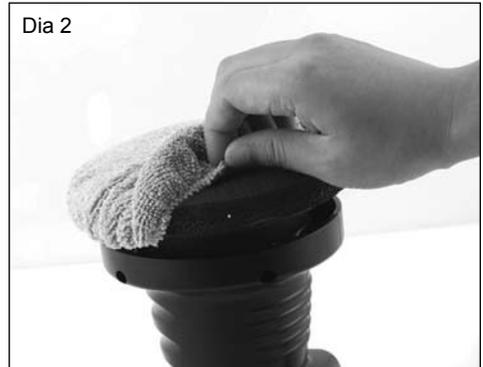
2. Spread a tablespoonful of polish evenly over the surface of the cotton pad (dia 3). Do not apply polish directly to the car.
