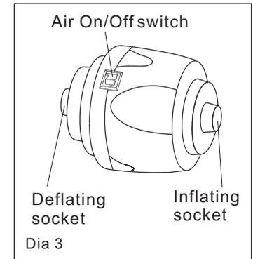
3. Insert cigarette plug into the 12V output socket on the jumpstart (item 2) or other equal source then press the Air on/off switch on the Inflator/Deflator body at I position to start inflating/deflating.
